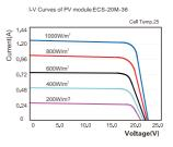
I-V Curves of PV module ECS-20M-36 at various cell
